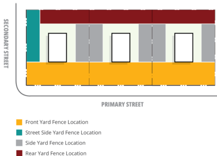
Figure 1 Lot Fence and Wall Configuration
